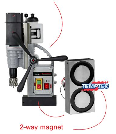
The 2-way magnet saves energy when the machine is not being used. The machine sticks sufficiently at half the magnetic force, this ensures you use less energy. The magnet generates less heat which makes the lifespan of the machine is longer. Only with full magnetic force the machine can be used for drilling.
